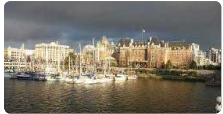
New developments should respond to the surrounding architectural context of the Inner Harbour as defined by street walls, facade rhythm and horizontal cornice lines (as illustrated above).
