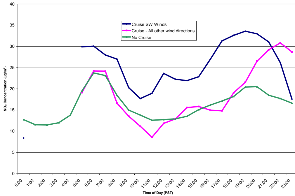
Figure D.17: Diurnal Weekday Variation in Average NO 2 Concentrations Segregated by Wind Direction at Victoria Topaz: May - September, 2008
